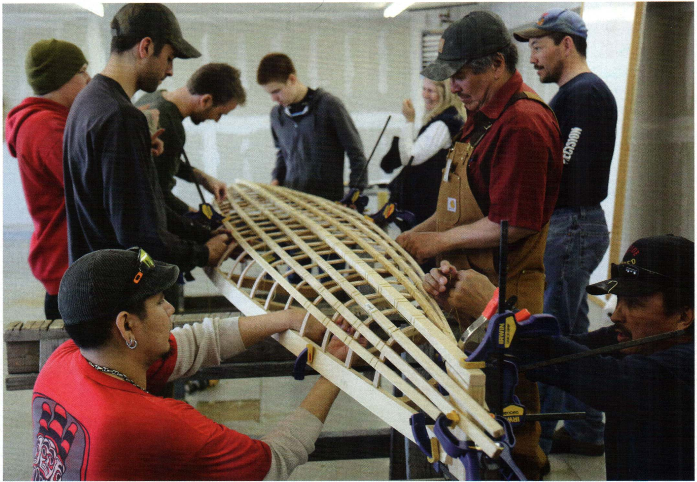
Students lash together a qayaq frame in a class taught by Greenlandic champion Maligiaq Padilla.
